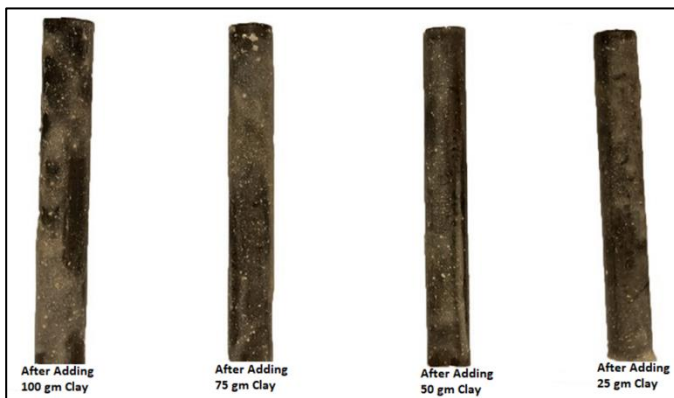
Fig. 6: Clay accretion profile in WBM with FR
