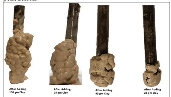
Fig. 5: Clay accretion profile in the basic WBM
